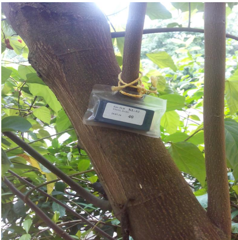
Figure1: An outdoor TLD deployment for Environmental Gamma Radiation Monitoring
